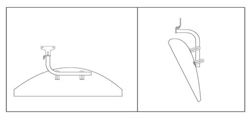
Brackets can be mounted on top or inside fenders.
